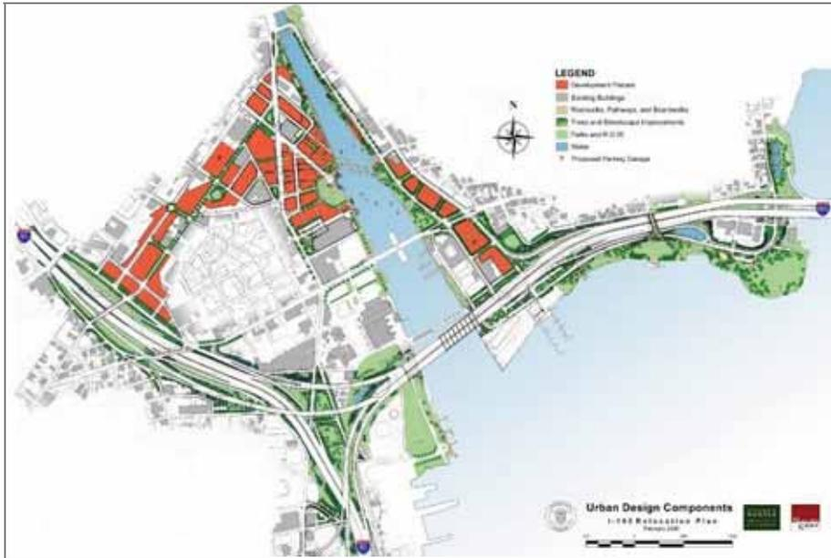
The design incorporates numerous pedestrian amenities, including walkways along the Providence River, and allows much greater access to the waterfront. The design also includes a new signature – or landmark – bridge.
