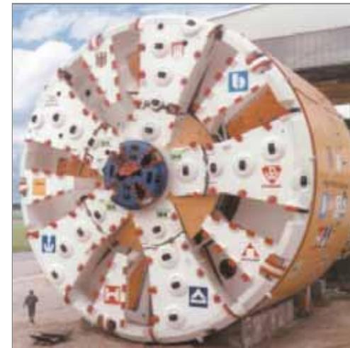
German Tunnel Boring Machine – 46 feet in diameter
