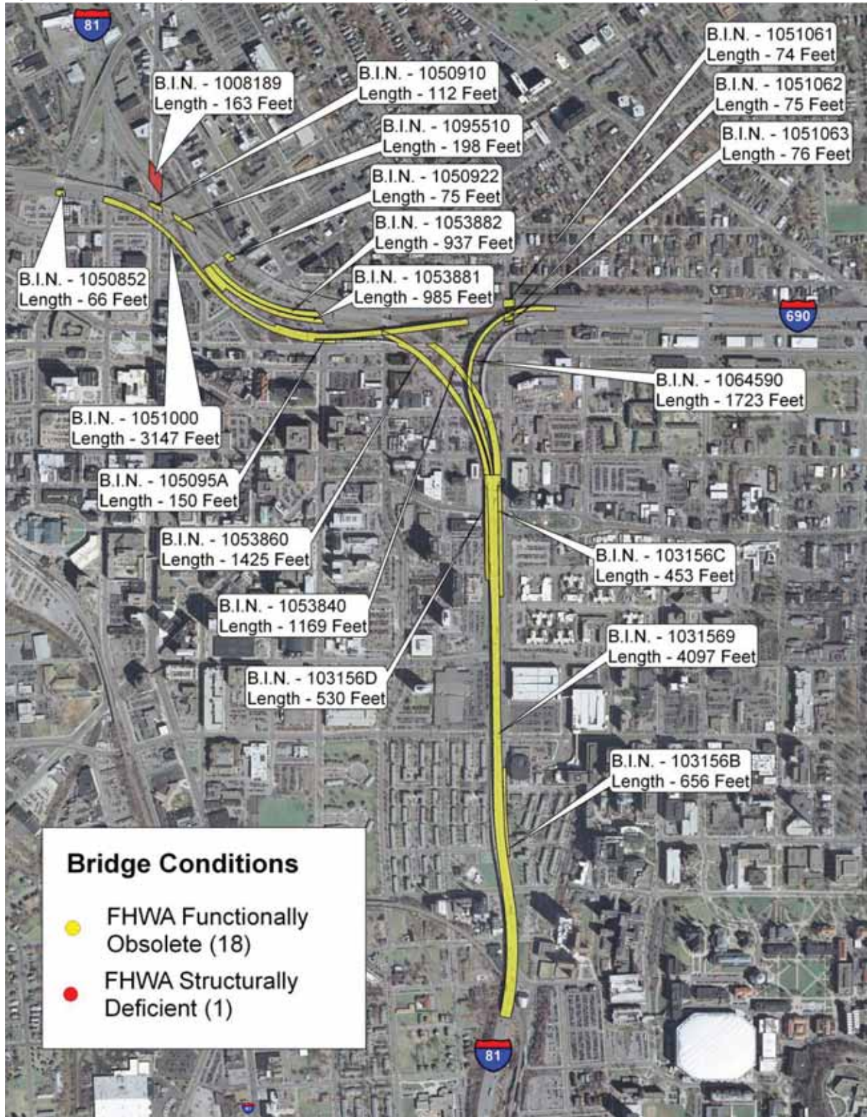
Figure 6 – Structurally Deficient and Functionally Obsolete Bridges in the Viaduct area
