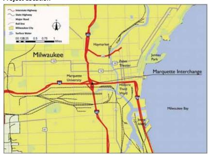
This project involved the complete reconstruction of the interchange of I-94, I-794, and I-43 in downtown Milwaukee, the "Marquette Interchange." The interchange was aging, and had an outdated design that did not function well for high traffic volumes merging and weaving at high speeds. In addition, the physical presence of the elevated interchange resulted in
