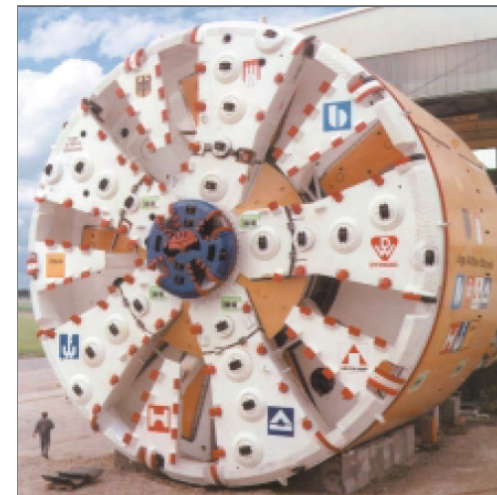
German Tunnel Boring Machine – 46 feet in diameter
