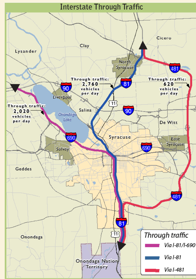
Of the 44,000 vehicles per day observed on I-81 south of the southern I-481 interchange (Exit 16A), only about 12% travel through the Syracuse region on the interstate system without stopping. Approximately 6% (2,760 vehicles per day) of these 44,000 vehicles per day take I-81 from I-481 on the north to I-481 on the south or vice versa. Another 5% (2,020 vehicles per day) use I-81 to access I-90 via I-690 and only about 1% (620 vehicles per day) currently use I-481 to travel through the region.
